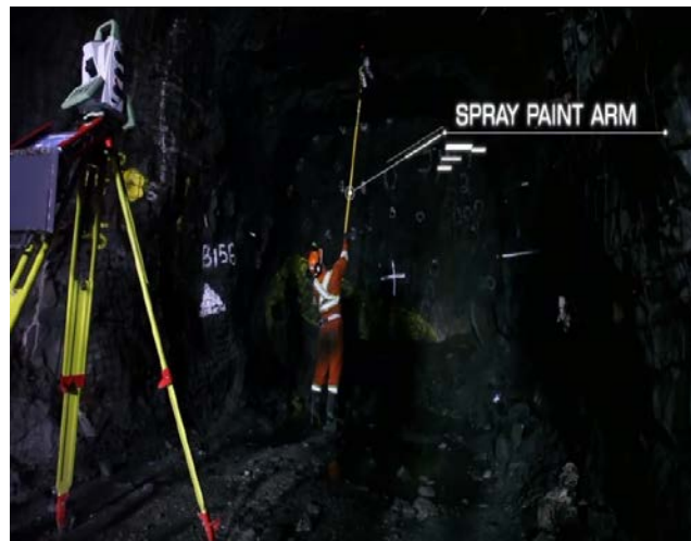
Figure 8. Crankline being marked on back
