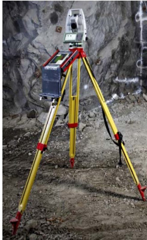
Figure 1. MOSS Components: As shown above, the tablet is contained in a durable hard-shell cover that which provides additional protection against drops while making it more portable.
