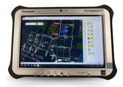
With MOSS implemented in active headings, we see a direct result of improved workflows and faster cycle times. MOSS is able to capture and provide solutions for: comparison between mine design and actual blast, setting of line and grade, collar drill hole location, 3D drill pattern generator, face scanning/photos, and cavity monitoring. The entire seven-step process takes on average 10-20 minutes which is dependant on the experience level of the user.
